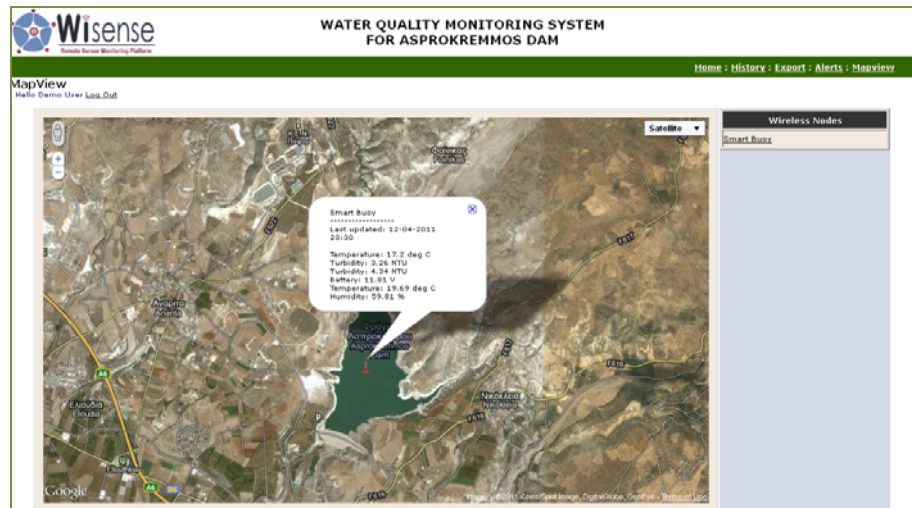
Figure 9. Real Time Data from Asprokremmos Dam using Wisense remote monitoring Platform
