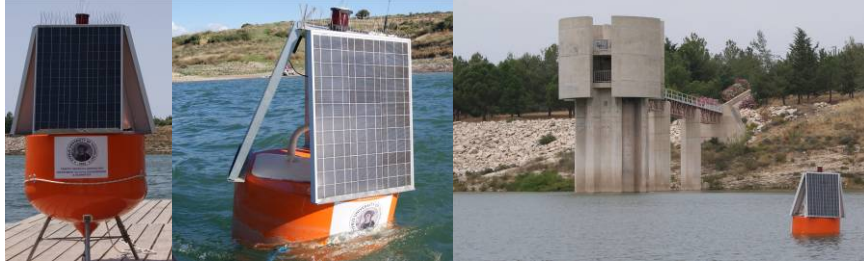
Figure 3. Pictures of smart sensor platform deployed in Asprokremmos Dam
