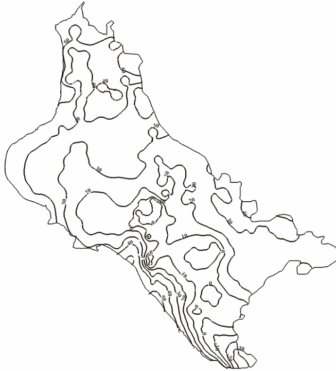
Figure 3. Hydraulic heads counters of aquifer for year 2012.
