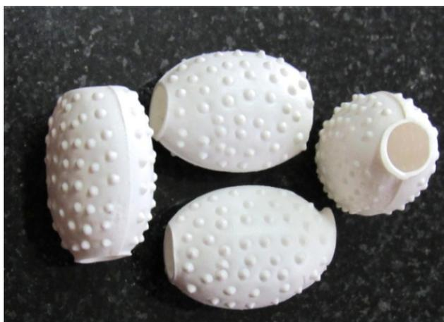
Figure 2. Photo of plastic biofilm support carriers used in biological reactor
