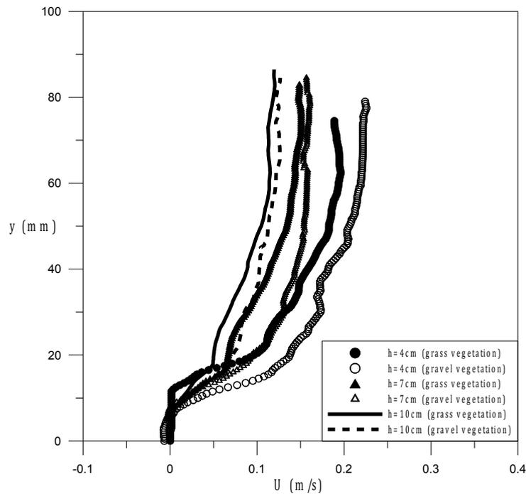
Figure 3. The effect of permeable bed on the velocity distribution. Vegetation height and discharge are constant and equal to  $2\text{cm}$  and  $0.970\text{lt/s}$ .
