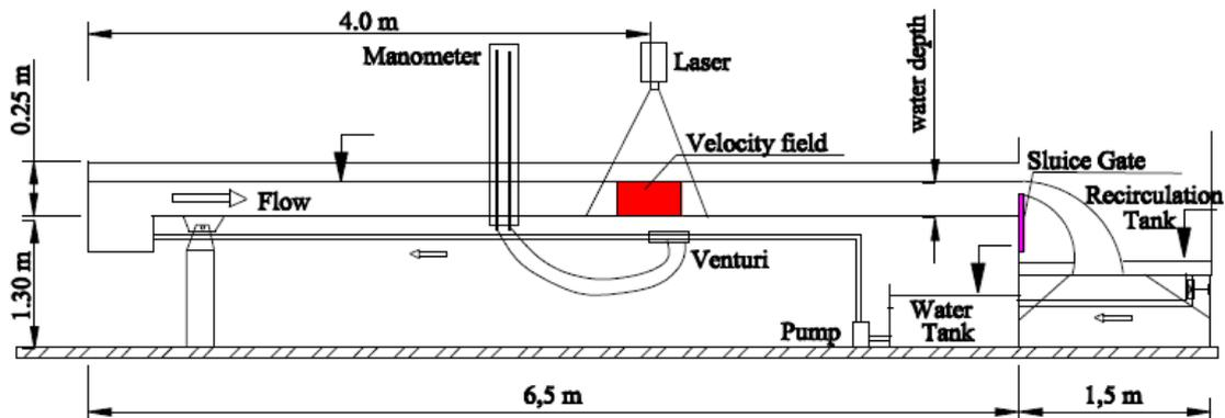
Figure 1. Experimental apparatus.
