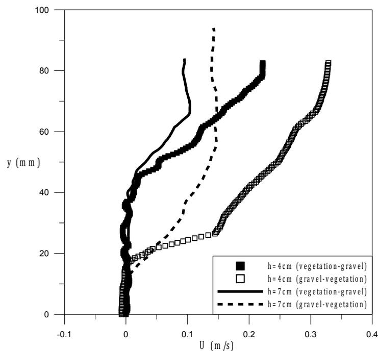
Figure 4. The effect of transition from vegetated to gravel bed and vice versa on the velocity distribution. Vegetation height and discharge are constant and equal to 2cm and 0.970lt/s.
