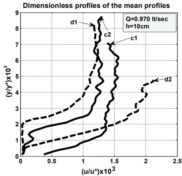
Figure 6. Dimensionless velocity profiles (c and d).
