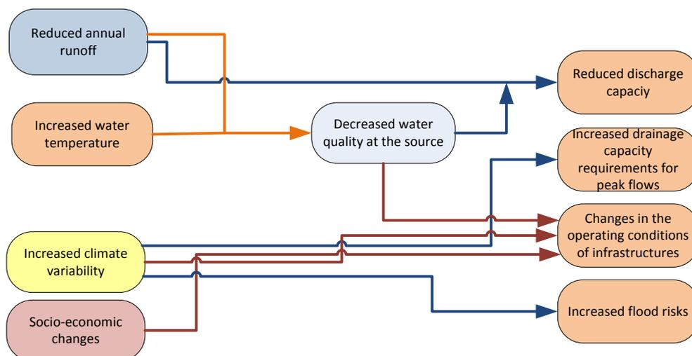
Figure 2. Impacts of climate change on waste water drainage and treatment systems
