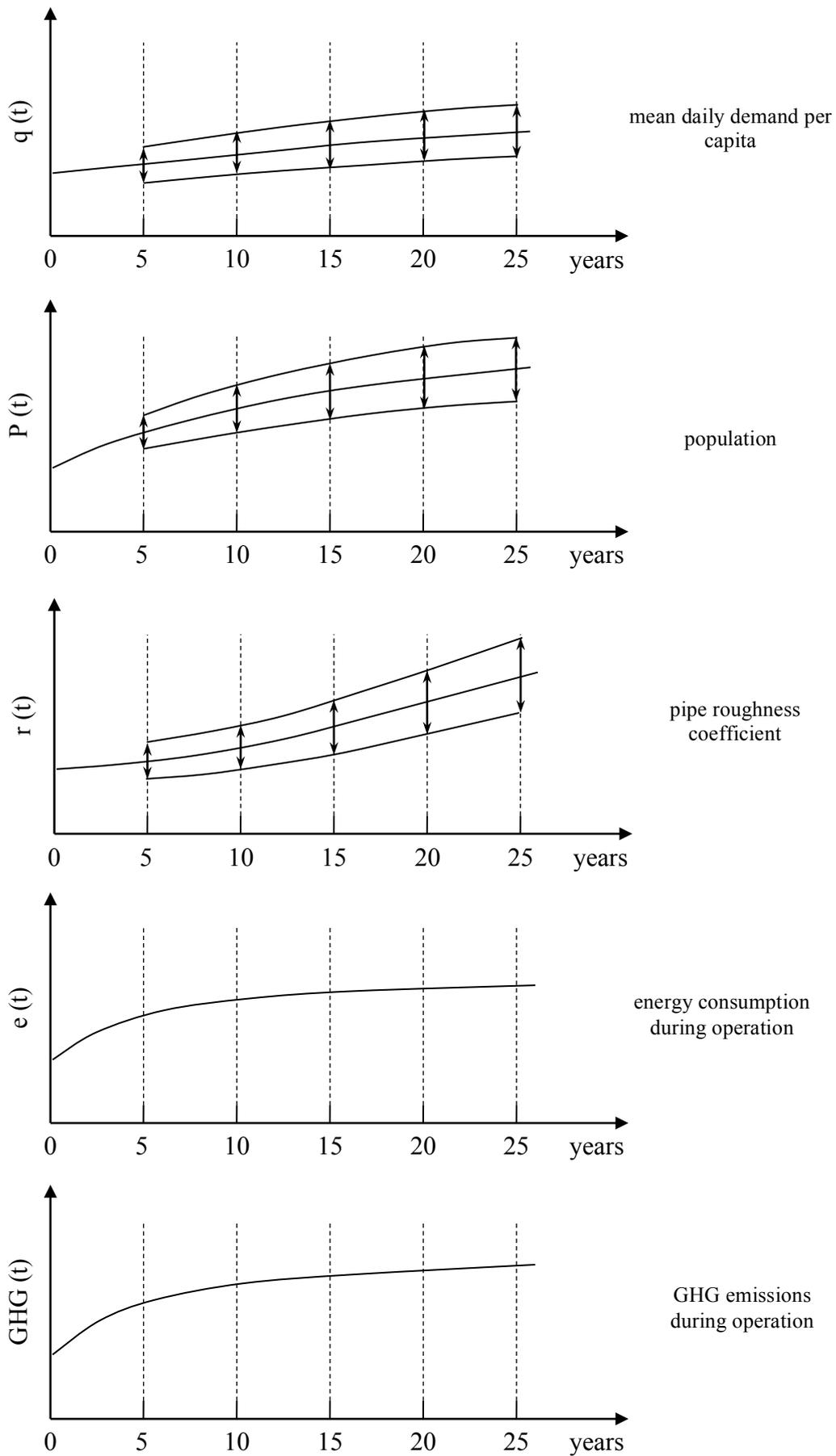
Figure 1. Indicative time dependence of some important parameters in the design of a municipal water supply and distribution system.
