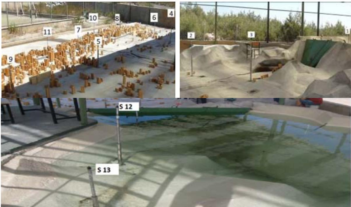
Figure 9. Water level sensors in downstream area (upper) and in the reservoir (bottom).
