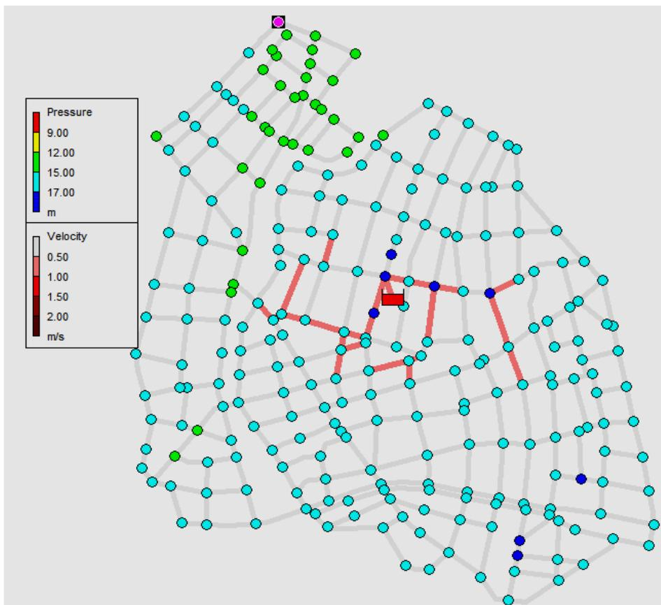
Figure 3: Pressure and velocity distribution of Scenario 3
