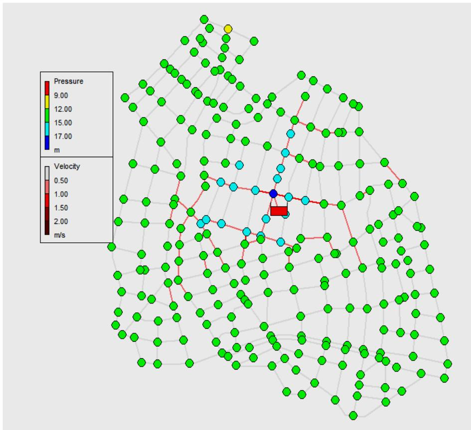
Figure 2: Pressure and velocity distribution of Scenario 2
