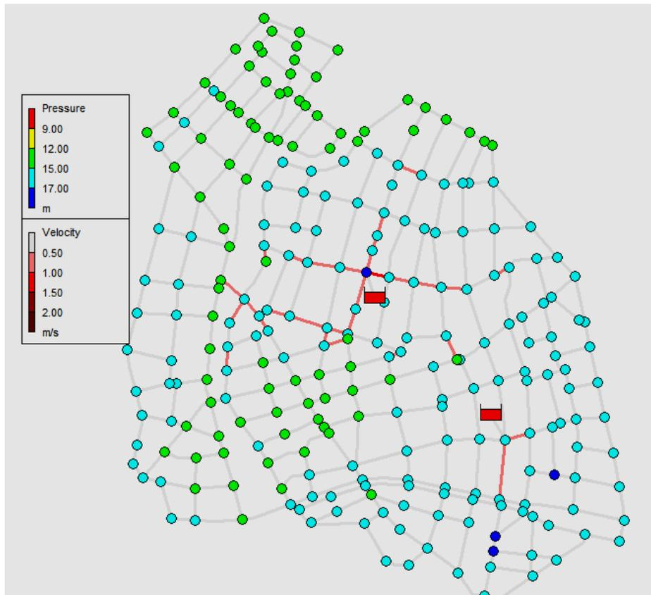
Figure 4: Pressure and velocity distribution of Scenario 4
