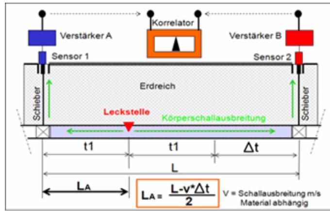
Figure 9. Localization of leaks.
