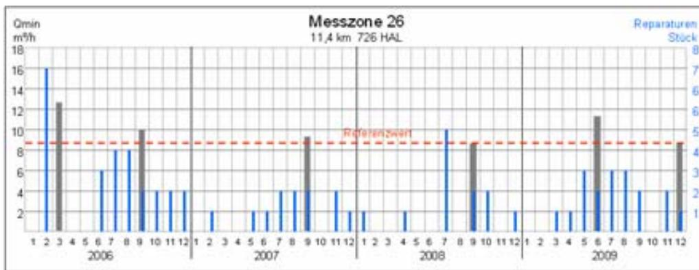
Figure 7. Documentation of the results of zone measuring over 4 years (inflow quantity and damages).
