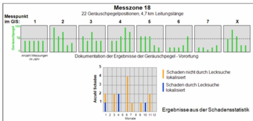
Figure 8. Documentation of results of the acoustic sound logger and damages in one measuring range.
