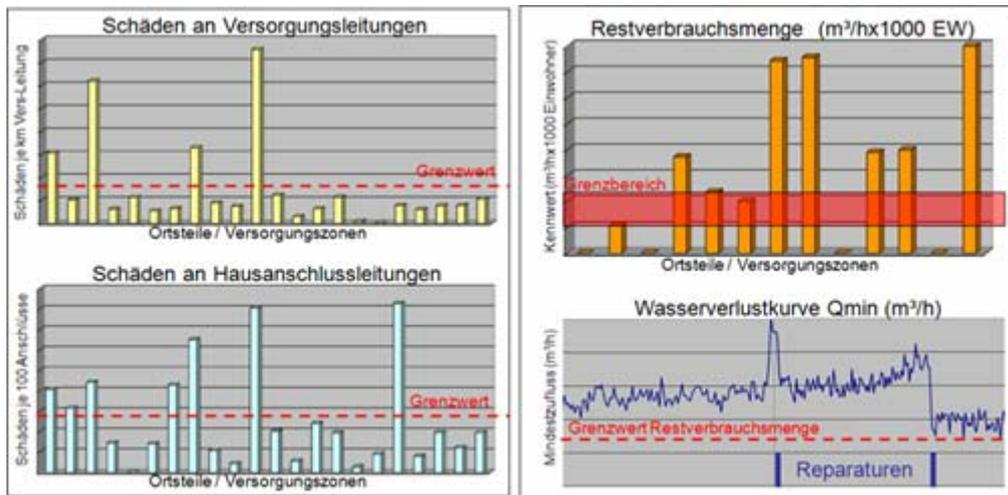
Figure 10. Damage evaluation in measuring areas: damages on main pipes, damages on service pipes (left). Rest consume quantity in measuring areas; Record of the minimum inflow with points of repairs (right).
