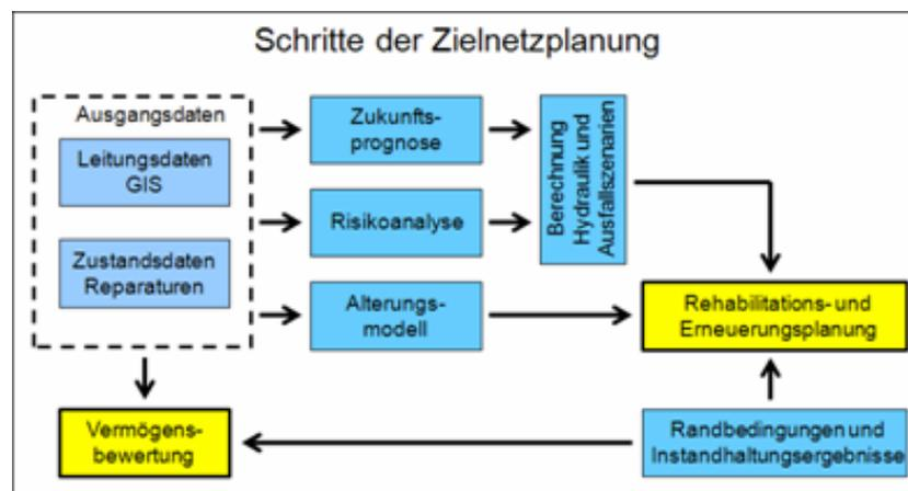
Figure 4. Steps of the “target system planning”.
