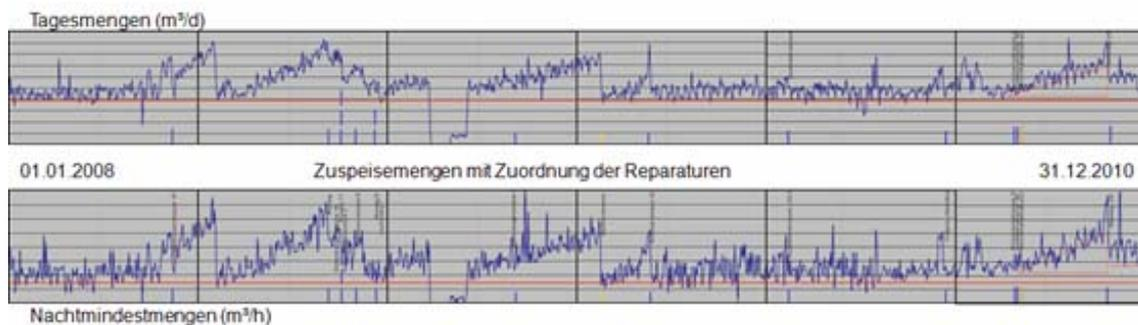
Figure 6. Records of the inflow monitoring over 3 years ( $Q_d$ ,  $Q_{min}$ ).
