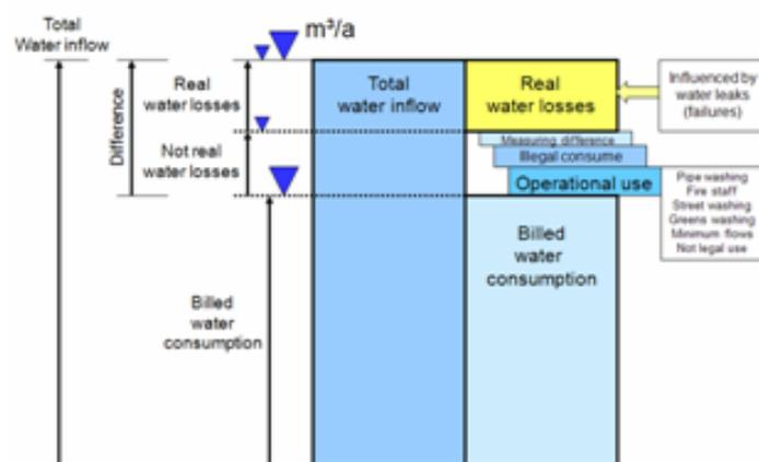
Figure 1. Calculation of water losses.
