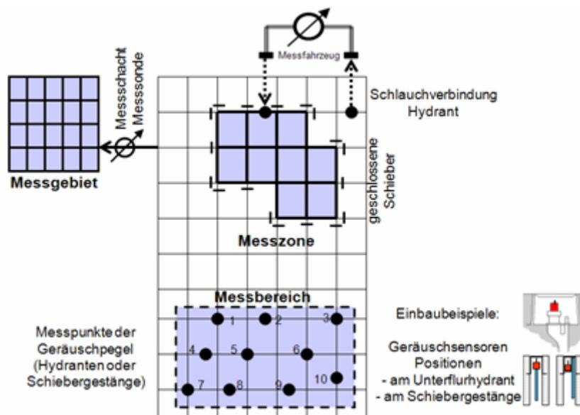
Figure 5. Schematic representation of monitoring system.
