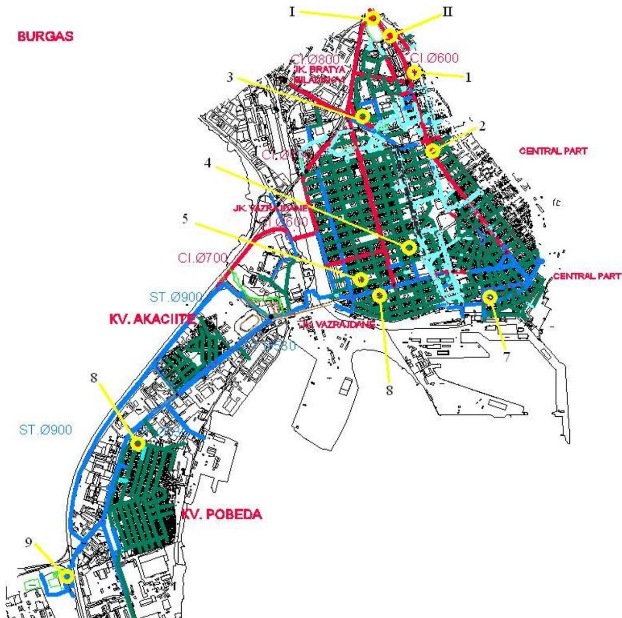
Figure 1. Situation of the surveyed water supply network in Burgas residential areas I and II – Measurement of water consumption, from 1 to 9 – measurement of water pressure
