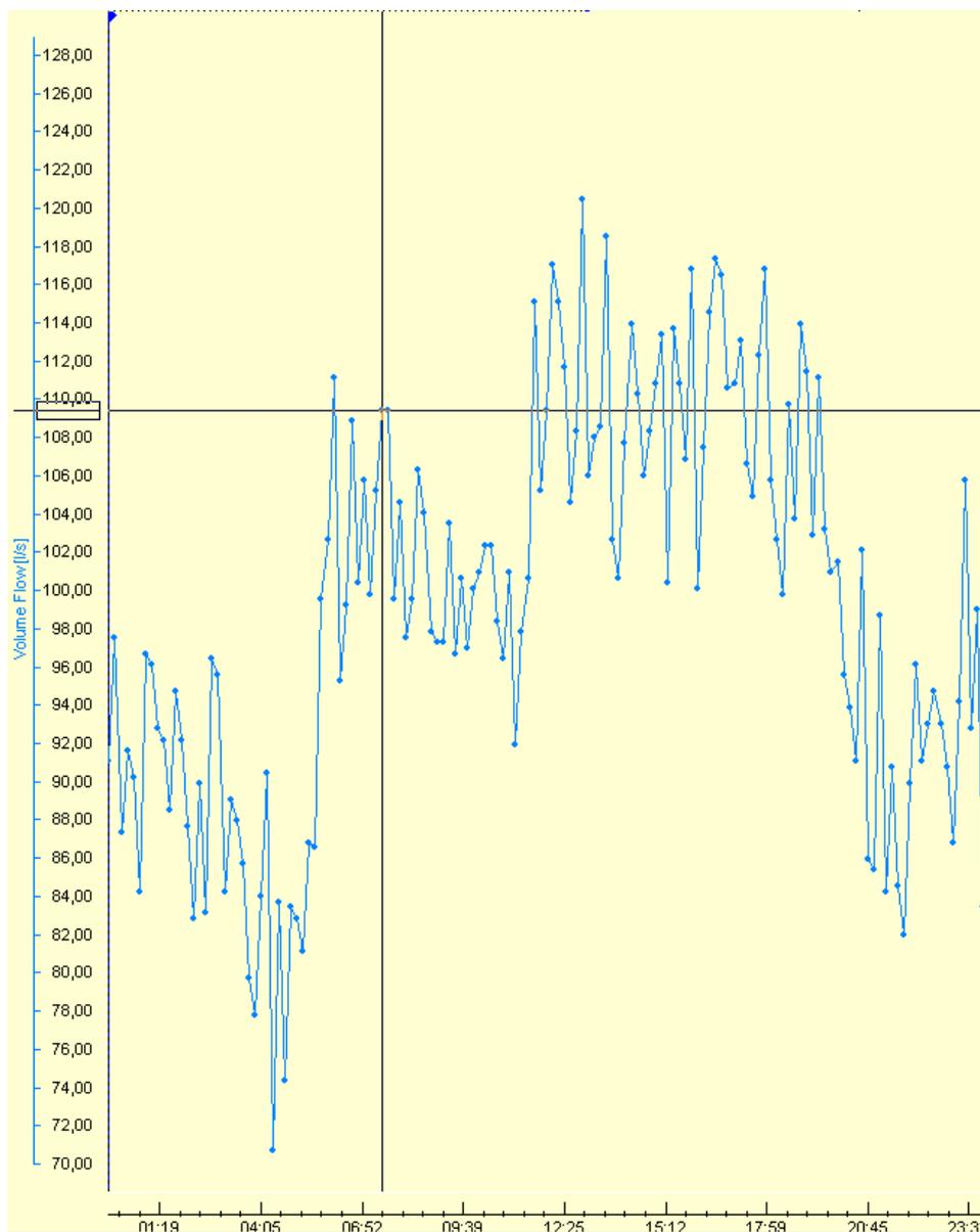
Fig. 5 Water consumption, measured on 16.07.2010 pipeline DN600, passing along Stefan Stambolov Str. (Fig. 1)
