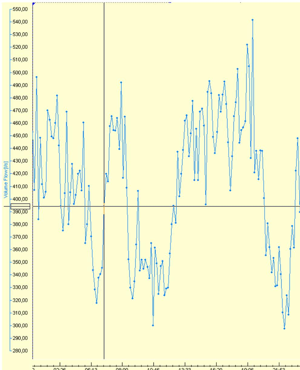
Figure 5. Water consumption, measured on 16.07.2010 pipeline DN800, passing along Struga Str. (Fig. 1)
