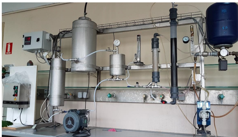
Figure 1. Catalytic ozonation continuous flow pilot unit
