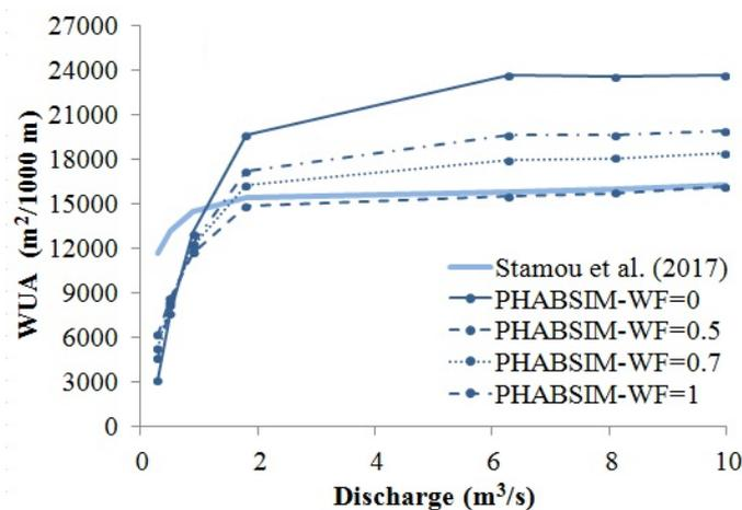
Figure 4. Variation of WUA with discharge and the Upstream WF for the Small Chub
