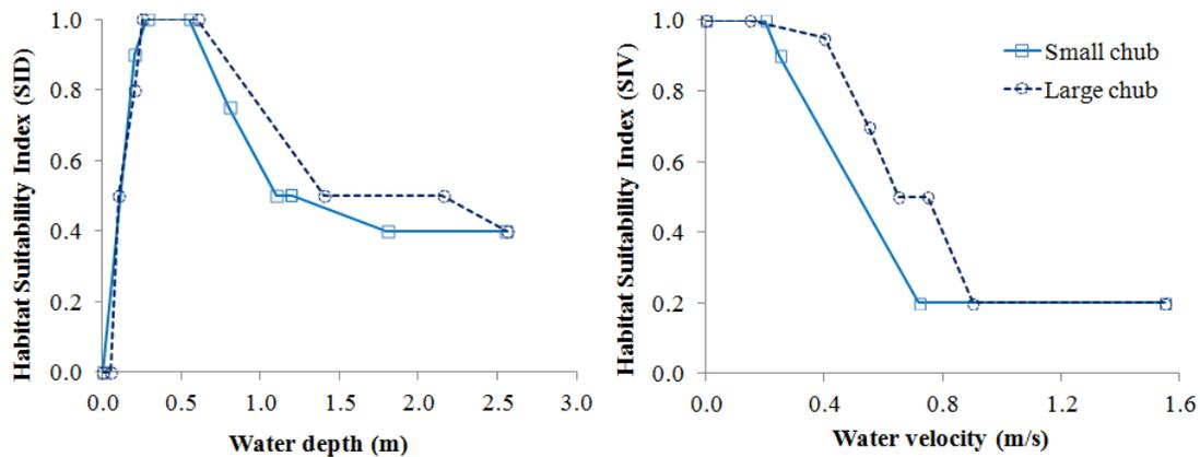
Figure 2. Habitat Suitability Curves for water depth and mean velocity by Stamou et al. (2017)
