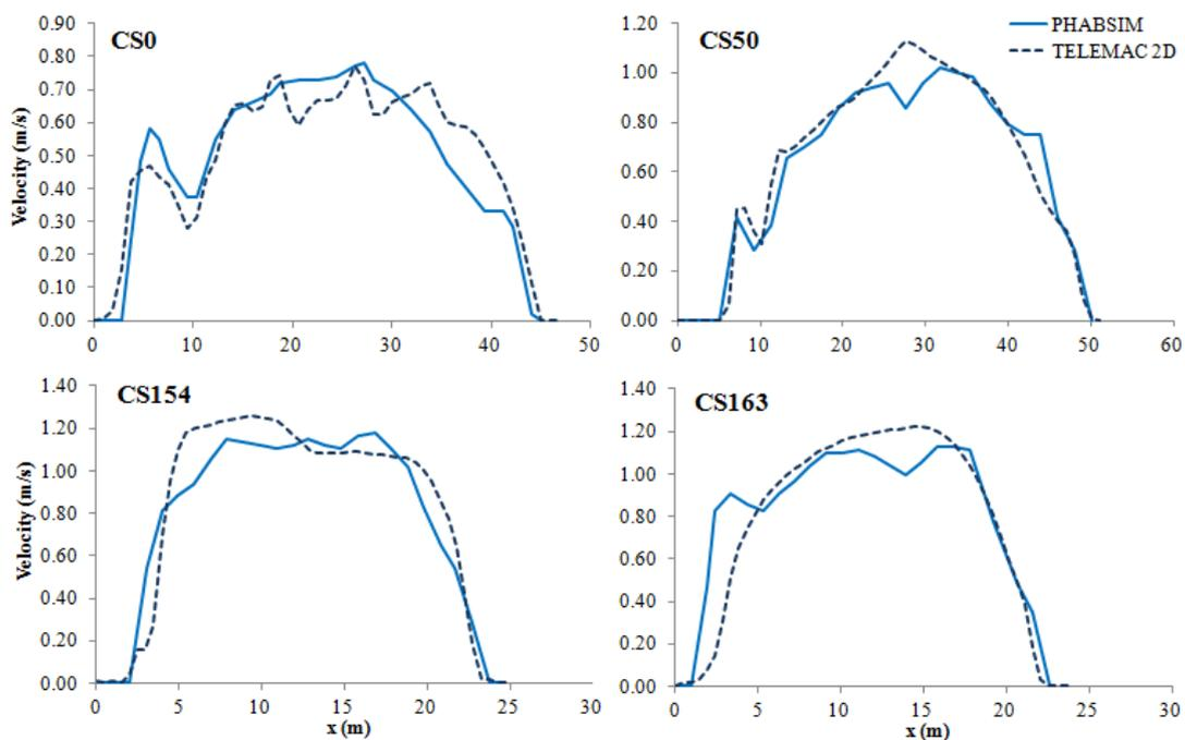
Figure 3. Velocity calculations by PHABSIM and TELEMAC-2D (Stamou et al., 2017) for  $Q=8.10 \text{ m}^3/\text{s}$
