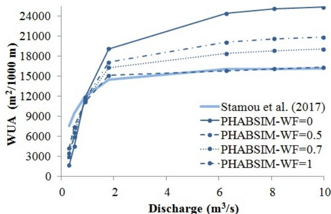
Figure 5. Variation of WUA with discharge and the Upstream WF for the Large Chub
