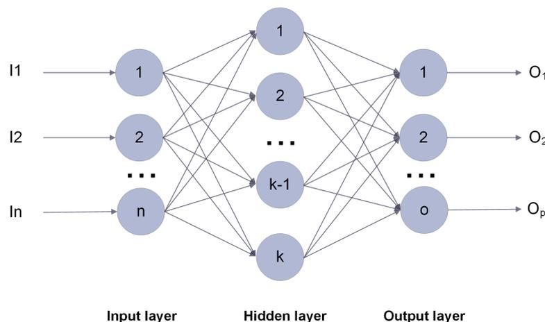
Figure 1. A typical feedforward neural network.  $n$  is the number of neurons in the input layer,  $k$  is the number of neurons in the hidden layer and  $o$  is the number of neurons in the output layer.
