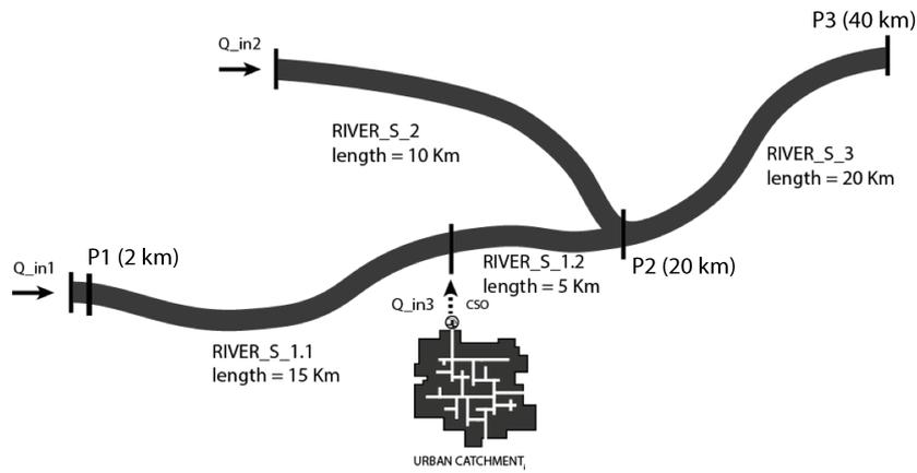
Figure 1. Synthetic set-up of the hypothetical case-study: Experiment 1 attends only to the main river section (S\_1.1, S\_1.2, S\_3) and Experiment 2 is composed by the full set-up.
