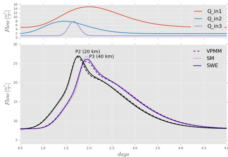
Figure 3. Routing in Experiment 2. Above is shown the 3 input hydrographs. Below the flow propagated at 2 sections of the river (corresponding to P2 and P3).
