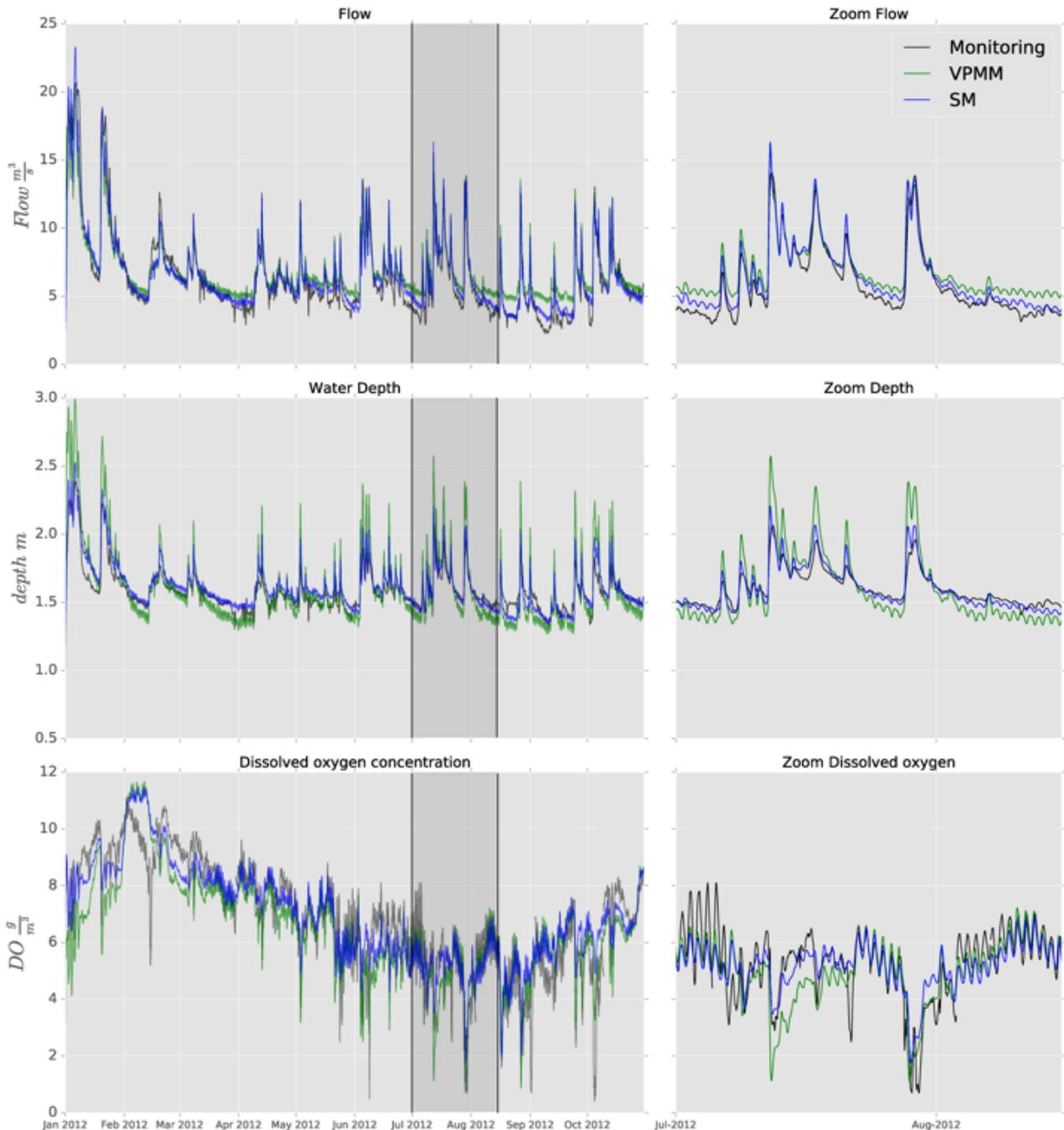
Figure 4. Comparison of monitoring data, VPMM and SM simulations for flow, water depth and dissolved oxygen at the outlet of the Dommel catchment (~17 km downstream of the WWTP). In the left side: the dynamics for January to October of 2012. In the right side: a detail for two events between the 01-Jul-2012 and the 15-Aug-2012.
