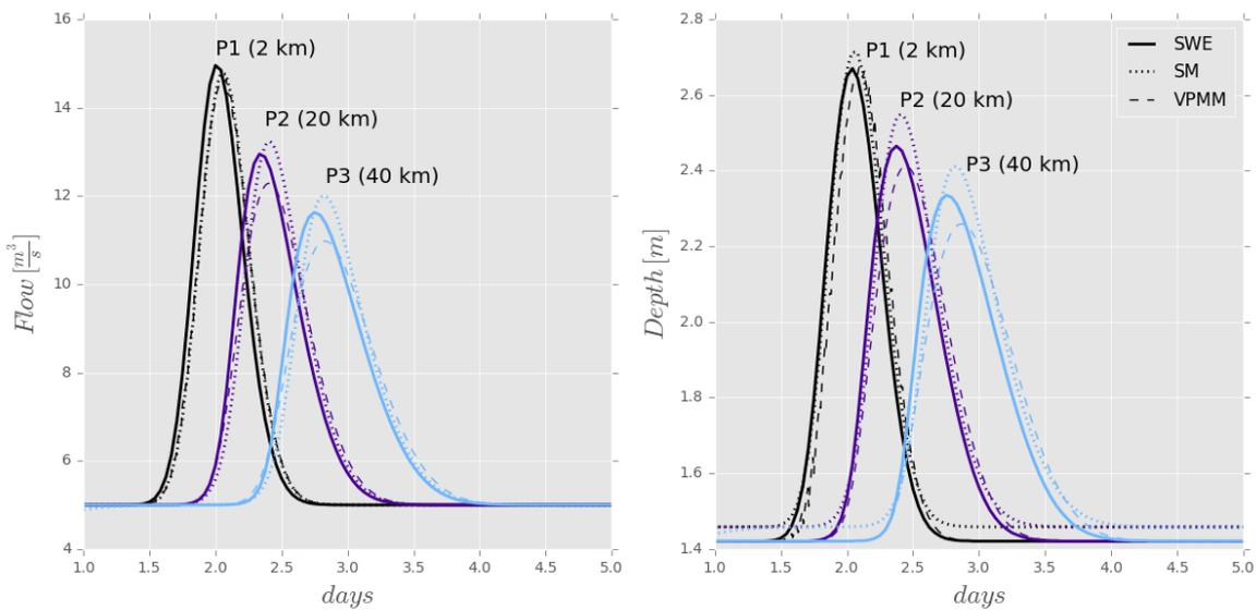
Figure 2. Comparison of flow and depth simulated at several locations along the channel (distances from channel's upstream boundary). Parameter combination E9 with 1000 m spatial discretization.
