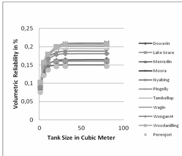
Figure 7: Volumetric Reliability for different Towns.
