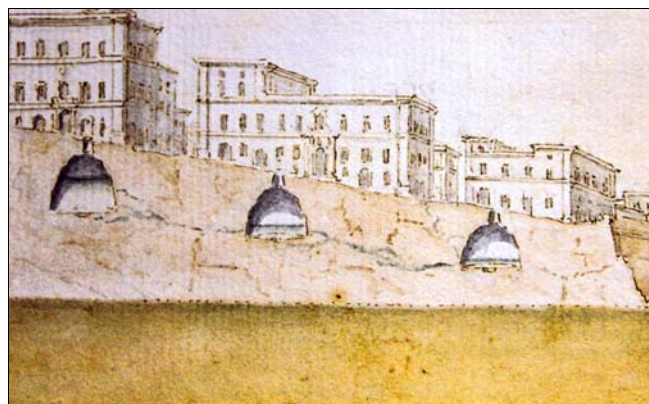
Figure 1: Illustration showing rock-hewn cisterns under the new capital city of Valletta (Spiteri, 2007)
